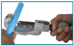
Step 1: Cutting the Tubes
